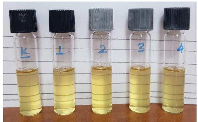
**Figure 1.** Mueller-Hinton broth containing tubes at the zero point of time. Tube 0 was assigned as control. The remaining Tubes 1-4 were respectively added with 1 to 4 drops CoQ10 containing eye drop.
